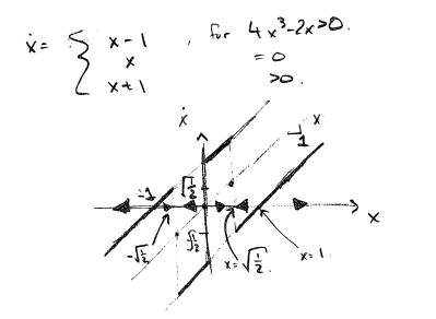
The closed-loop system has unstable fixed points at x = 0, x = -1, and x = 1.
